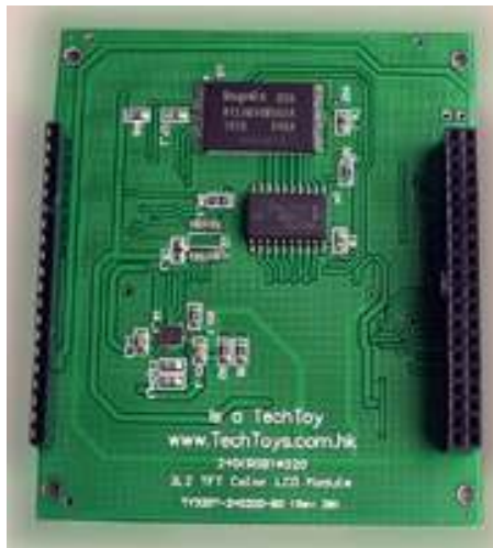
Fig. 3.10 – Display LCD e Touch Screen vista traseira, as conexões.
